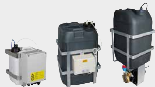
WASPT WASHER PUMP AND 5 OR 23 LITER TANK • Polyethylene tank with stainless steel cage • Delivery head: 5m (16ft), 11m (36ft) or 30m (98ft) • Versions with alarm for the lack of liquid in the tank • Also for third-party products • Operating temperature: from -10°C (14°F) up to +60°C (140°F) • Available voltages: 230Vac, 120Vac, 24Vac
